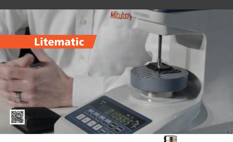
Mitutoyo's VL-50-B Litematic is a high-resolution digimatic measuring unit. The Litematic is ideal for measuring the thickness or height of a workpiece that can be easily affected by the measuring force.
